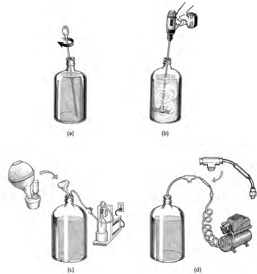
Figure 8.1: Degassing with a) a long mixing spoon, b) a lees stirrer, c) a Headspace Eliminator, and d) Gas Getter
